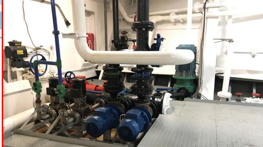
In front we will build up the cabinets Water intake from the sea chest
