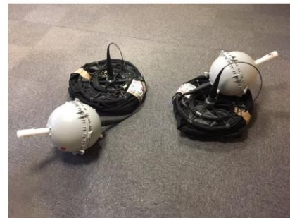
Temperature-measuring surface drifters. Credit: NEE
