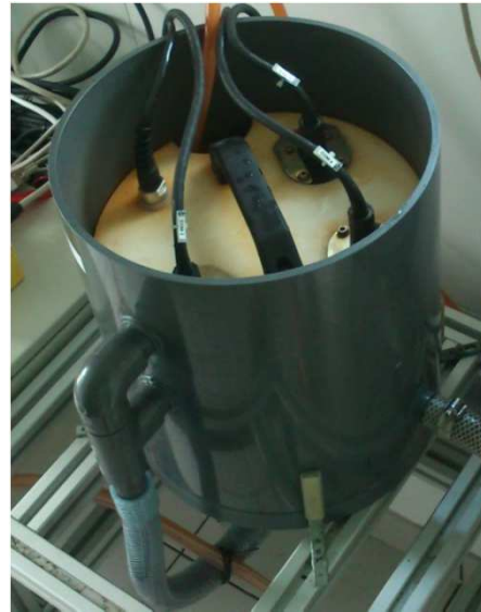
Sensors for Chl \alpha , phycocyanin, turbidity and oxygen
