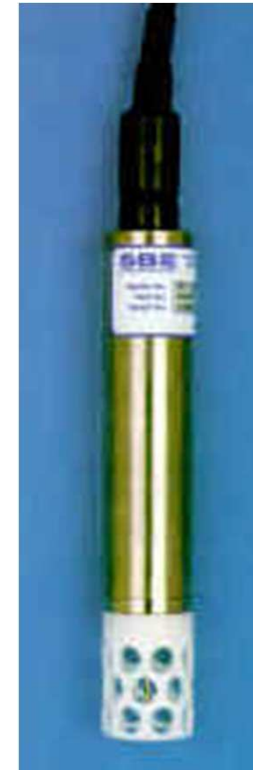
Thermometer SBE38 , at water intake
